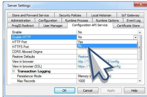
In the Configuration API Service Settings, input allow-listed domains into the **CORS allowed origins** setting.
